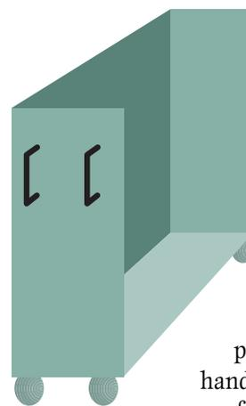
Handles should be located at the level of the load's center of gravity or slightly above. They should be spaced so that hands are directly in front of shoulders. This position provides optimal handling comfort and power for workers.
