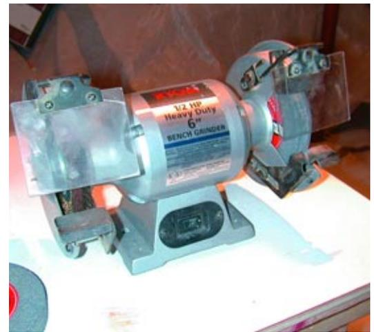
Tabletop and self-standing grinding wheels can be found in any section of work facilities. In many cases, the location was not chosen according to a work plan and unsupervised access is common, while safety rules are sometimes inexistent. Yet this location is a workstation and as such, should be governed by clear safety rules and closely supervised.
